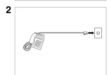
Plug a different regular telephone into the same telephone jack.
